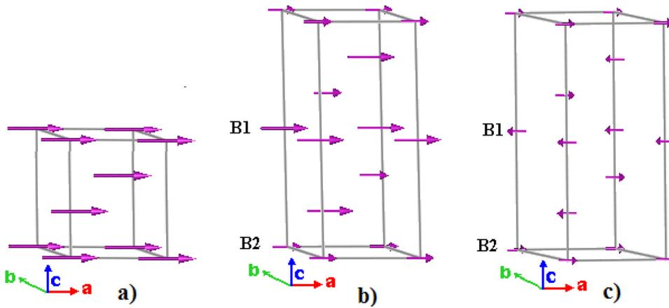
FIG. 1. Magnetic unit cells for the perovskite. Depicted magnetic unit cells are (a) ferromagnetic unit cell for 8% Ni, (b) the ferromagnetic (unequal moment magnitudes) doubled unit cell containing B1 and B2 layers for 21% Ni, and (c) the antiferromagnetic unit cell containing B1 and B2 layers for 31% Ni. The moment directions in the basal plane and labeling of B1 and B2 layers are arbitrary and chosen for convenience.
