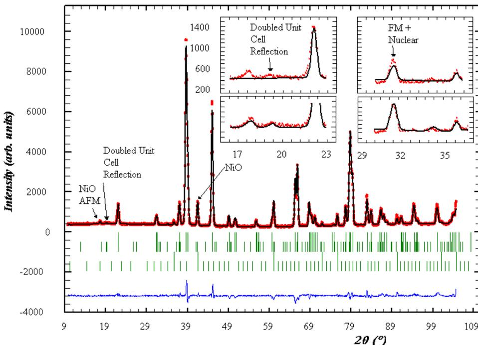
FIG. 3. Neutron-diffraction refinement of the  $\text{La}_{0.7}\text{Sr}_{0.3}\text{Mn}_{0.79}\text{Ni}_{0.21}\text{O}_3$  sample at 12 K (refined stoichiometric Ni content). The reflection markers below the plot are, in order, nuclear perovskite structure, ferromagnetic perovskite structure, NiO nuclear structure, and AFM NiO structure. The insets show the magnified regions around the small magnetic peaks prior to magnetic refinement.
