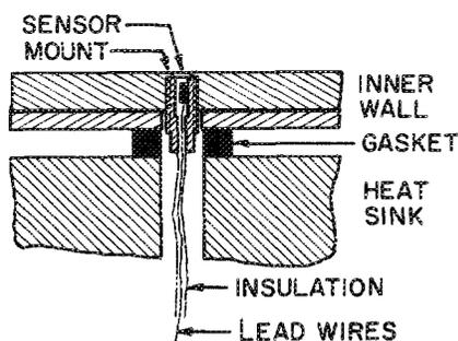
FIG. 4. Mounting of thermometers in chamber inner wall.
