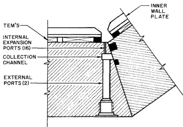
FIG. 5. Expansion manifold in chamber wall.
