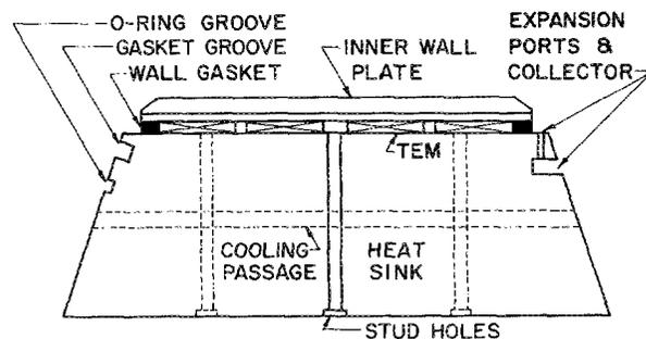
FIG. 3. Cross section of chamber wall.
