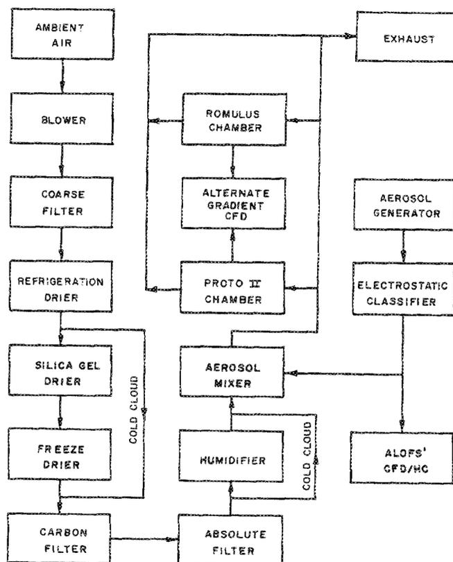
FIG. 1. Flow diagram of UMR simulation facility.
