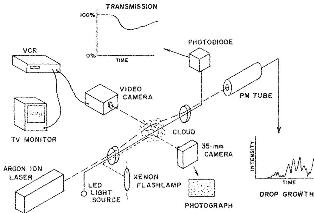
FIG. 6. Schematic view of optical systems.
