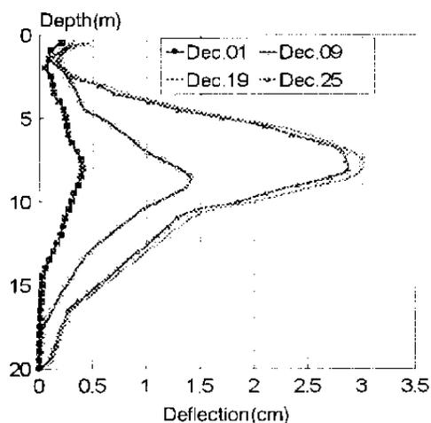
Fig.7 Deflection of soil around the pit(measured by No.3 inclinometer)
