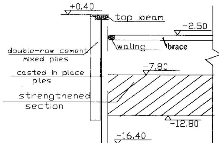
Fig.2 Cross-section of pit
