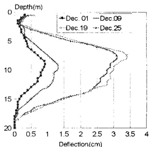
Fig.6 Deflection of soil around the pit(measured by No.2 inclinometer)
