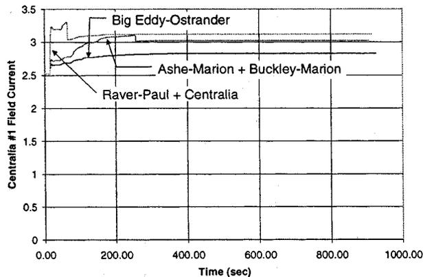
Fig. 6. Centralia-unit field current for the three outages.
