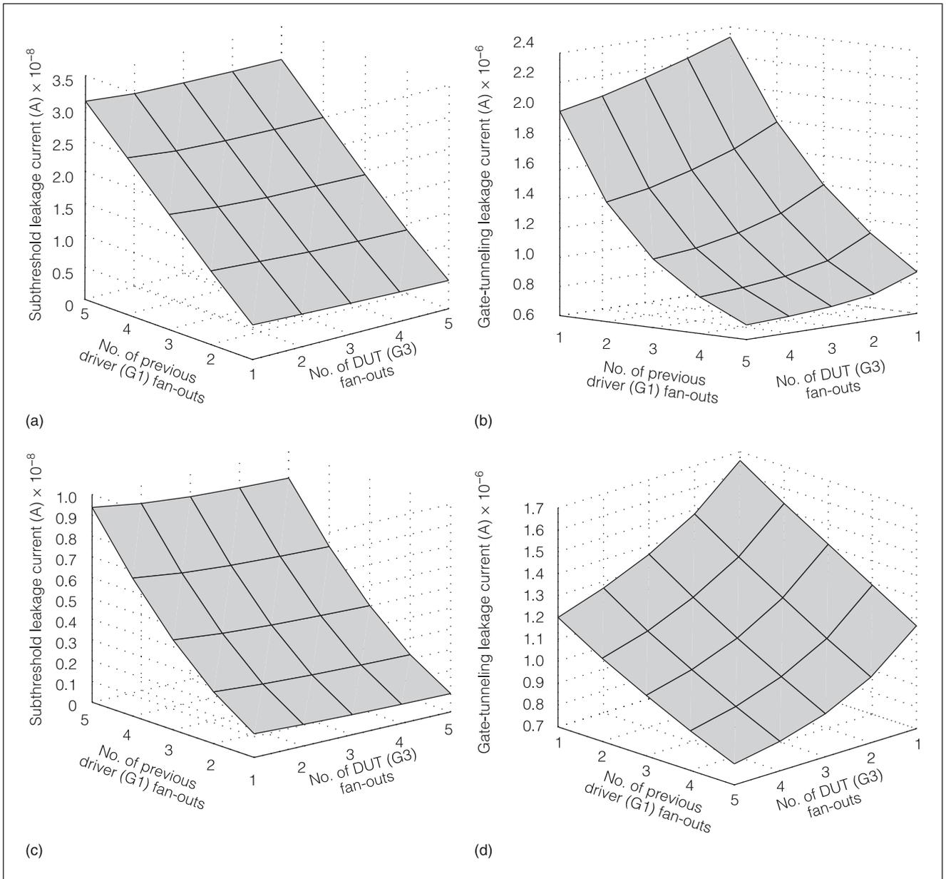
**Figure 6. Leakage current variation due to fan-out effect in BSIM4 45-nm technology: subthreshold leakage current with input 1 (a), gate-tunneling leakage current with input 1 (b), subthreshold leakage current with input 0 (c), and gate-tunneling leakage current with input 0 (d).**
