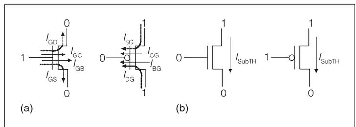
**Figure 2. The gate-tunneling and subthreshold leakage current in NMOS and PMOS transistors: maximum gate-tunneling leakage current state (a) and maximum subthreshold leakage current state (b).**
