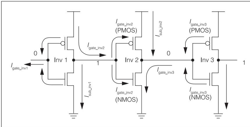
**Figure 4. Leakage current flows in nanoscale CMOS circuits.**
