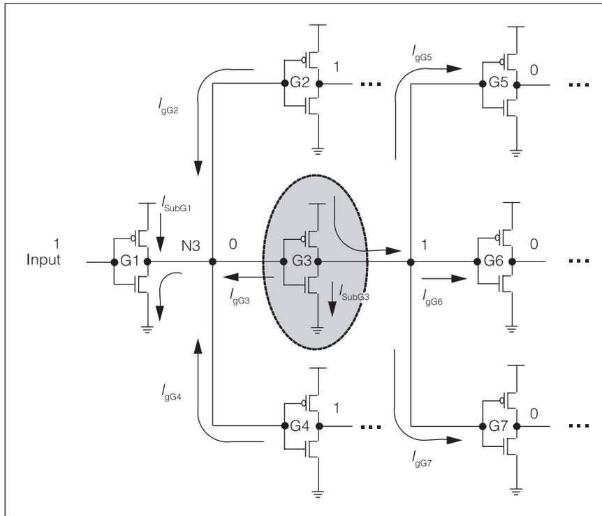
**Figure 5. Fan-out effect for the G3 gate. The leakage currents depend on the fan-out structures of the G3 gate. [W/L of PMOS is (90 nm)/(45 nm), and W/L of NMOS is (45 nm)/(45 nm), where W and L are the transistor channel width and length.]**
