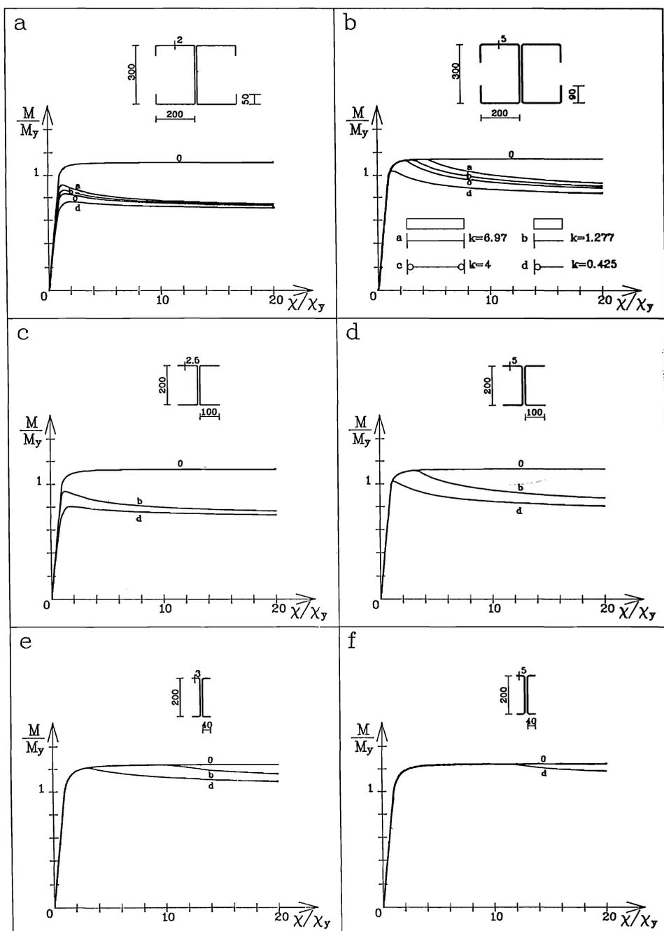
fig.2 - Influence of restrain conditions of flange
