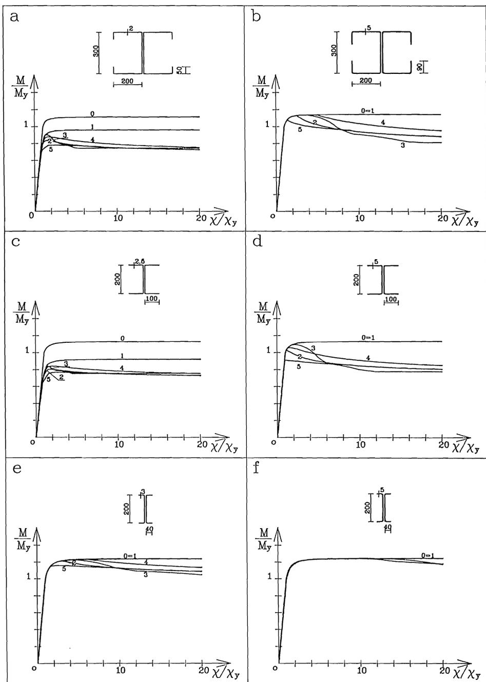
fig.1 - Influence of compressed flange instability model
