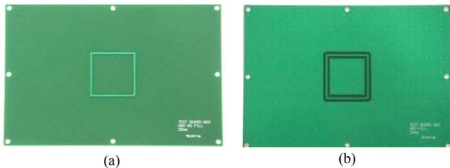
Fig. 4. Top view of test boards (a) 2-layer PCB without GND fill. (b) 2-layer PCB with GND
