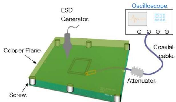
Fig. 2. Experimental setup for induced voltage measurement
