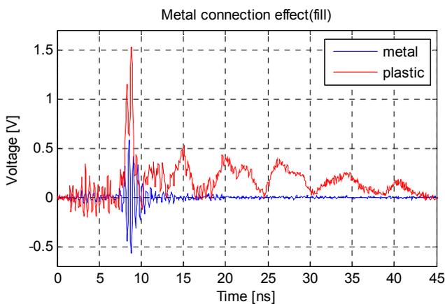
Fig. 8. Comparison waveform of measured induced voltage on trace, placing metal screws and plastic screws
