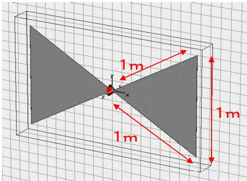
Figure 15. Butterfly Antenna Used for Far-field Measurement
