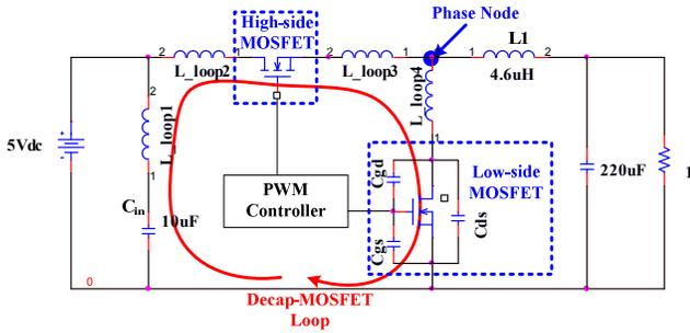
Figure 2. Synchronous Buck Converter with Parasitic Elements
