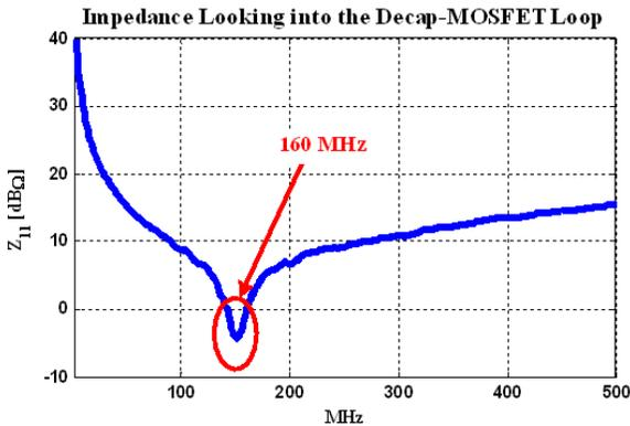
Figure 7. Impedance Looking into the Decap-MOSFET Loop
