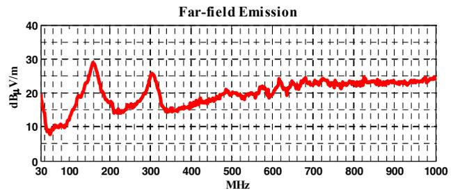
Figure 1. Far-field Emission of a Synchronous Buck Converter
