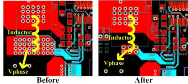
Figure 13. Reduction of the Exposed Phase Voltage Area
