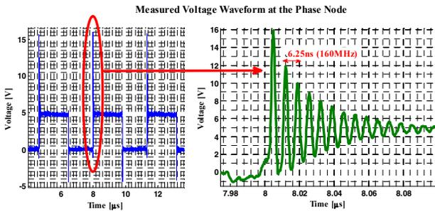
Figure 3. Measured Voltage Waveform at the Phase Node
