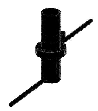
Fig. 4. Main shaft and tunnels' mesh.
