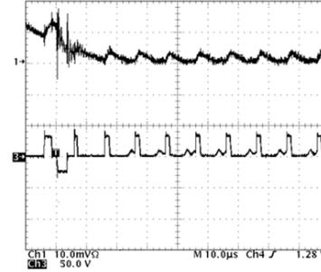
(b) Load step-down change at non-peak inductor current.
