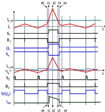
Fig. 7. Switching sequence of proposed controller.
