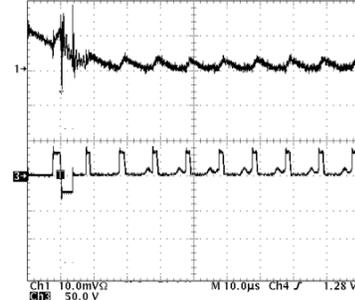
(a) Load step-down change at peak inductor current.
