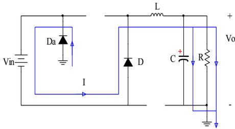
Fig. 3. Equivalent circuit for load step-down transient operation.
