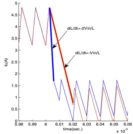
Fig. 12. Inductor current for worst case of dynamic response.
