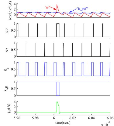
Fig. 8. Control logic with transient control.
