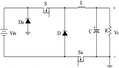
Fig. 1. Diagram of a buck derived dc-dc converter.
