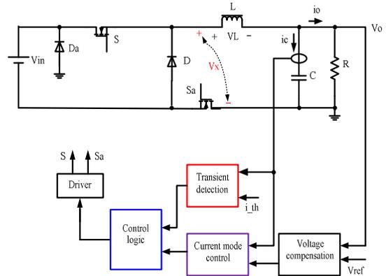
Fig. 4. Principle of the proposed controller.
