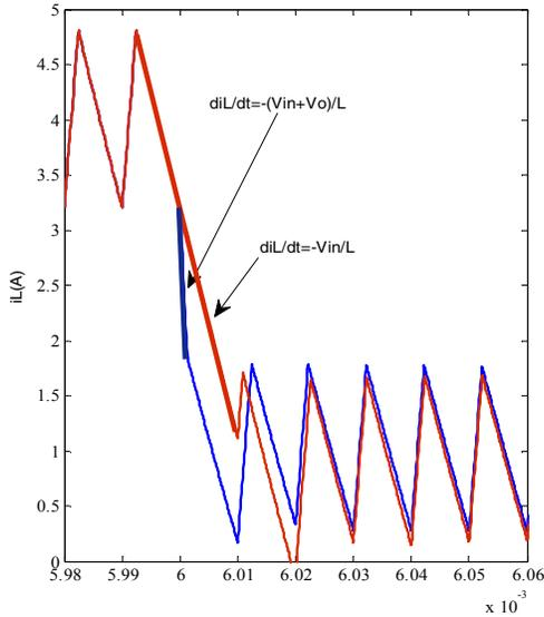
Fig. 10. Inductor current for best case of dynamic response.
