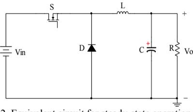
Fig. 2. Equivalent circuit for steady-state operation.
