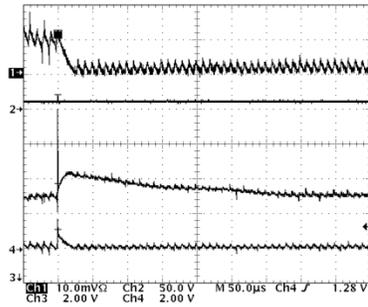
(a) Load step-down change at peak inductor current.
