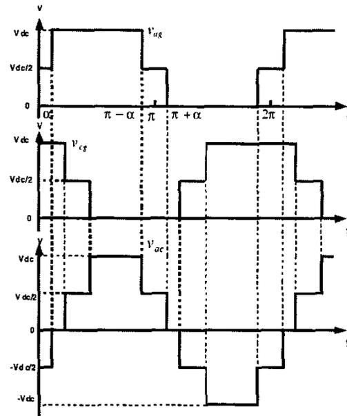
Figure 7. Staircase control of the bulk inverter.
