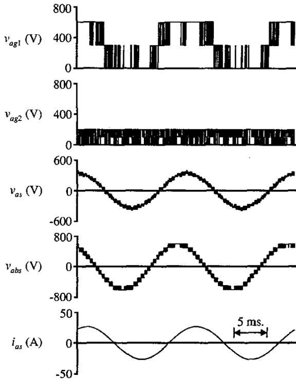
Figure 6. Cascade-3/3 inverter simulation results.
