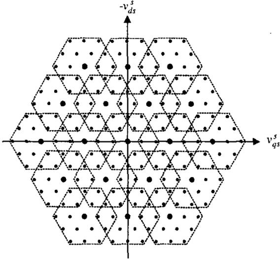
Figure 3. Cascade-3/3 vector plot for maximal distortion.
