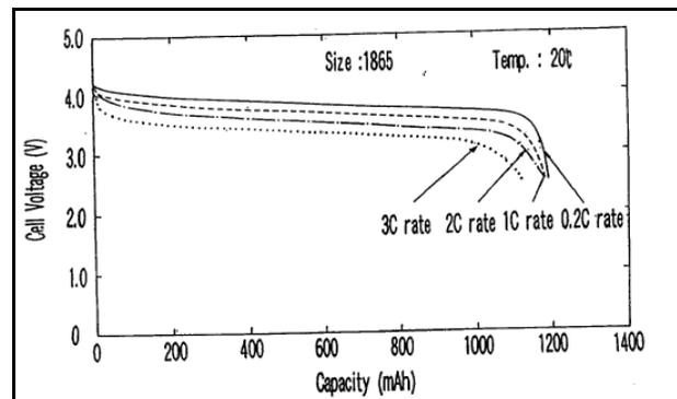
Fig. 7. Discharge characteristics of a Li-ion battery
