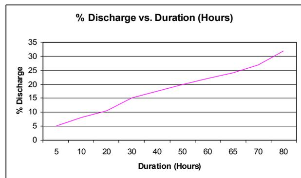
Fig. 6. Self-discharge of NiMH battery stored at 100% SOC
