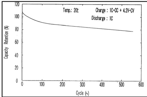
Fig. 9. Cycle characteristics of a Li-ion battery
