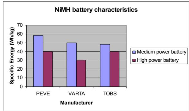
Fig. 2. Specific energy comparison of high and medium power NiMH batteries by various manufacturers
