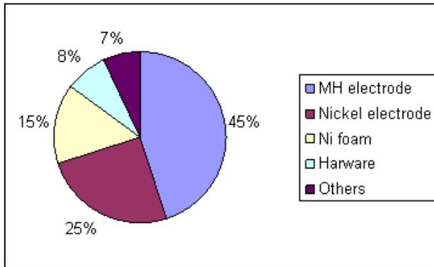
Fig. 11. Cost distribution of NiMH battery components
