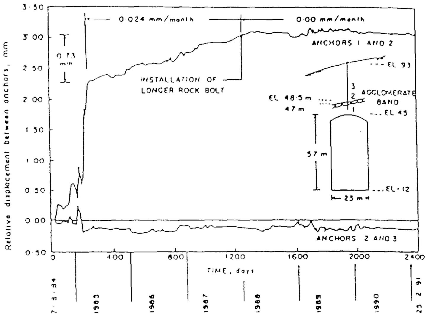
Fig. 3 Monitoring of Agglomerate Band by MPBX in Powerhouse Cavern of Sardar Sarovar Project Gujrat, India (Goel et. al.)
