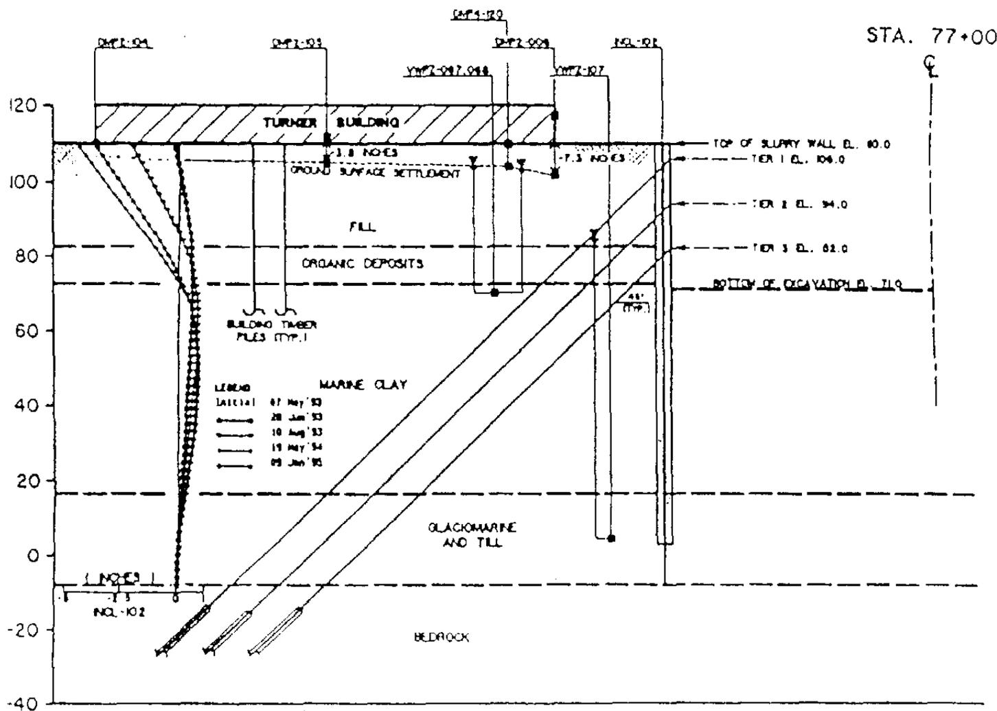
Fig. 2b Deformations at Station 77+00, Slurry Wall (Vaghar and Bobrow)
