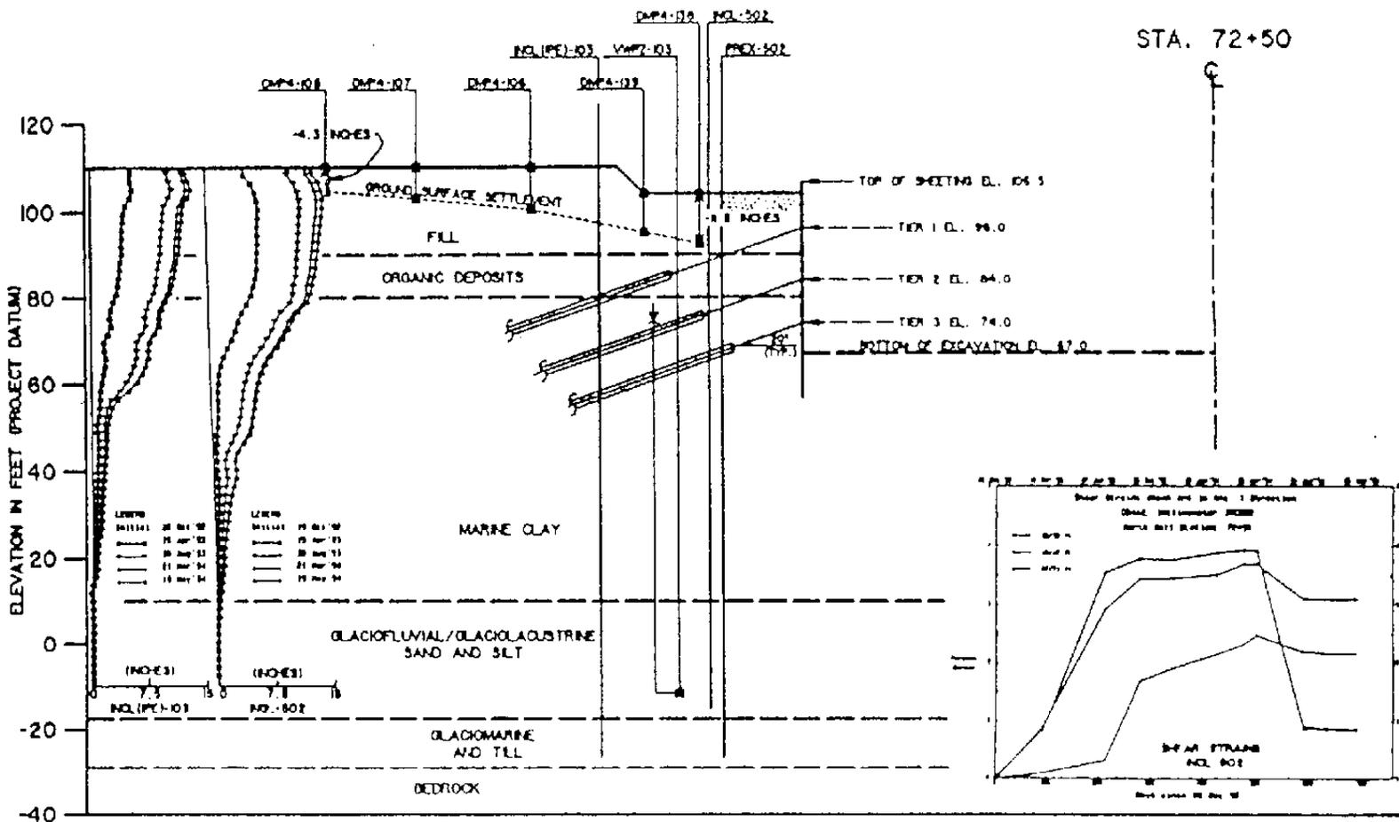
Fig. 2a Deformations at Station 72+50, Sheet Pile Wall (Vaghar and Bobrow)
