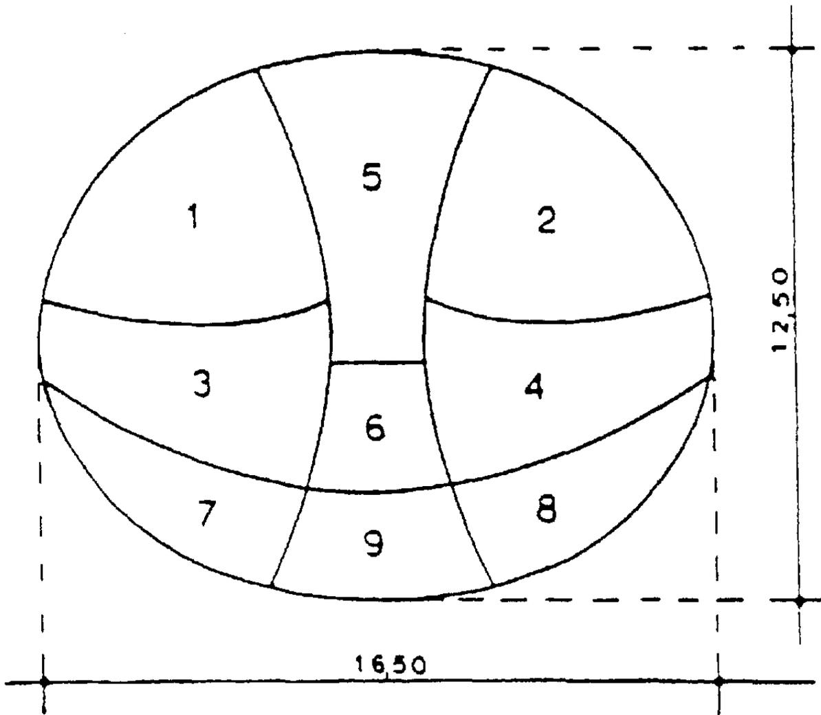
Fig. 1 Station Geometry and Excavation Stages (Kavvadas)
