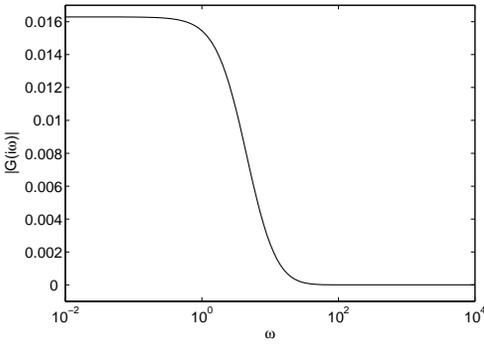
Figure 4. The magnitude of the transfer function of the convection diffusion system given in (16) evaluated at  $s = i\omega$  for  $10^{-2} \leq \omega \leq 10^4$ . The integrals are computed exactly and 40 terms are taken in the infinite sum.
