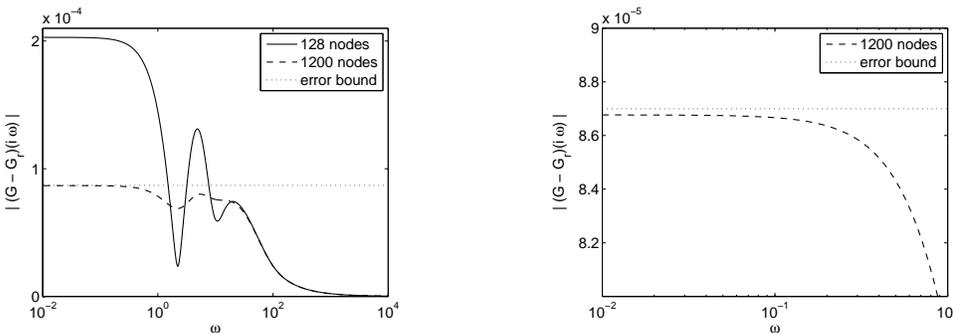
Figure 6. Balanced POD transfer function error  $|G(s) - G_r(s)|$  for  $r = 3$  evaluated at  $s = i\omega$  for  $10^{-2} \leq \omega \leq 10^4$  using 128 and 1200 nodes (left) and the same plot over the range  $10^{-2} \leq \omega \leq 1$  (right).
