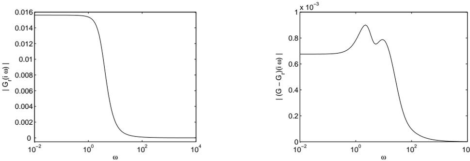
Figure 5. Magnitude of the balanced POD transfer function  $|G_r(s)|$  for  $r = 2$  (left) and transfer function error  $|G(s) - G_r(s)|$  (right) both evaluated at  $s = i\omega$  for  $10^{-2} \leq \omega \leq 10^4$ .
