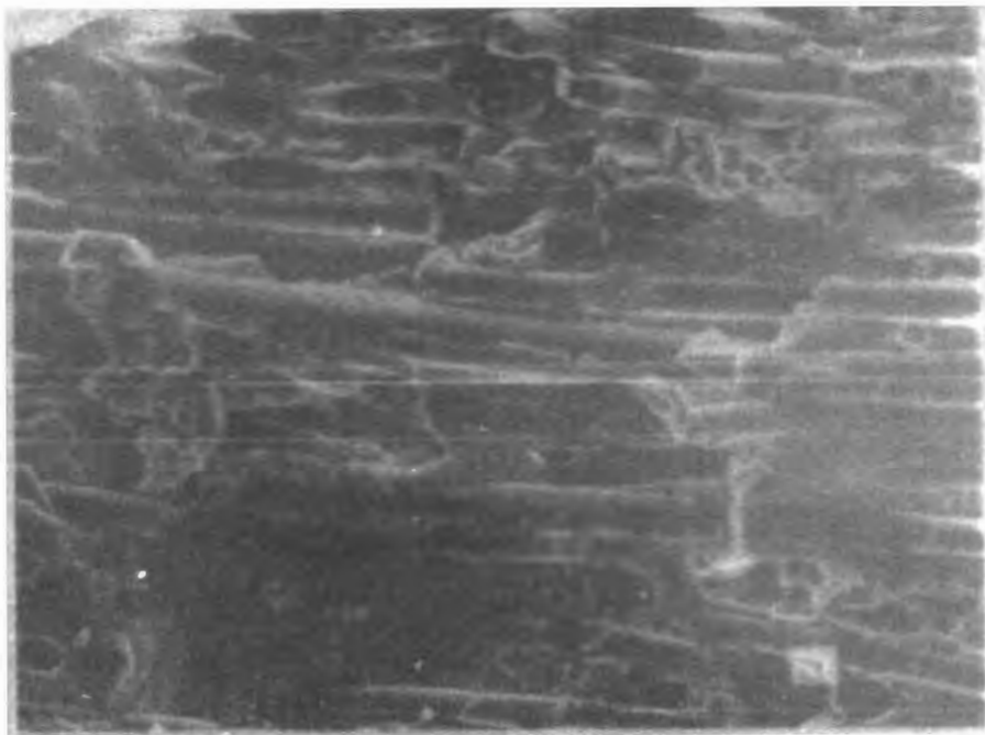
Fig. 33. SEM fractograph of YAS-7 containing boron nitride coated Nextel 440 fiber, hot pressed in argon at 1100C, showing varying degrees of fiber/matrix bonding.
