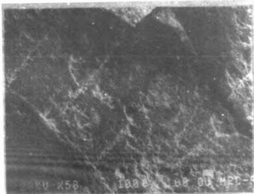
Fig. 20. SEM photomicrograph of a hot pressed surface of unidirectional carbon fiber reinforced cordierite matrix showing regularly spaced matrix microcracks perpendicular to the fiber direction.
