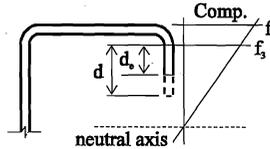
**Figure 1 - Unstiffened Element Subjected to a Stress Gradient**
