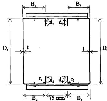
**Figure A.1 - Waterloo Test Specimen Cross-Section[6]**
