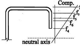
Figure 2 - Edge-Stiffener Stress Position Comparison
