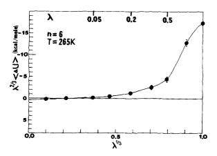
FIG. 2. Plot of  $\lambda^{2/3} \langle \Delta U \rangle$  vs  $\lambda^{1/3}$  for a monolayer cluster of n=6 water molecules on the model AgI basal substrate at 265 K. C(6) is -3/kT) times the area under the curve drawn through the data points (4).
