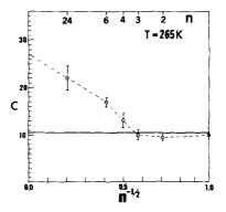
FIG. 3. C vs  $n^{-1/2}$  for T=265 K. The uncertainties indicate the range in C obtained from the maximum and minimum areas under the curves indicated in Eq. (12). The solid line shows  $\ln(n/N_1^{p_0})=10.5$ . Its intersections with the data for C(n) locates an approximate value of  $n^*=3$ . The dashed line for n>6 indicates a possible straight line fit to the data for large clusters; the dot—dashed line guides the eye through the data points for small values of n.
