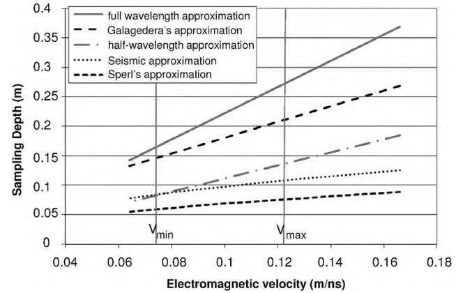
**Figure 5.** Analytical models predicting the sampling depth for 450 MHz GPR data over a range of electromagnetic velocity. The vertical gray lines show the minimum ( $v_{\min}$ ) and maximum ( $v_{\max}$ ) velocities observed in the 450 MHz data at the Mondavi site.
