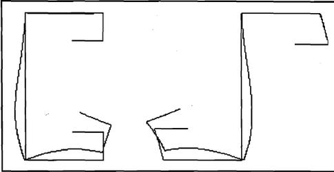
**Figure 4 Flange-lip distortional buckling mode**
