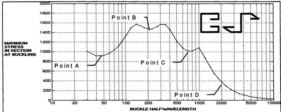
Figure 3 Buckling stress vs Half-wavelength for sections with deep lip stiffeners
