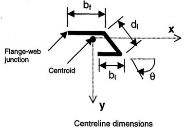
*Shear centre co-ordinates* of a compression flange with a simple lip and return lip (with slope =  $\theta$ ) are as follows:
