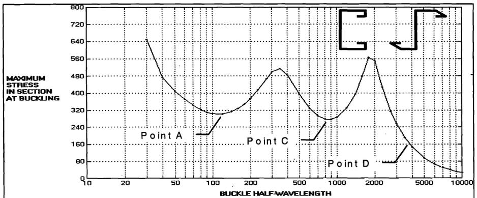
Figure 1 Buckling stress vs Half-wavelength for sections with shallow lip stiffeners
