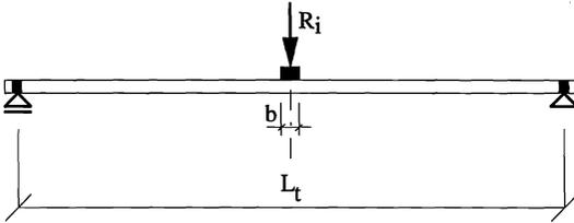
**Fig. 3.** Test set-up for internal support tests
