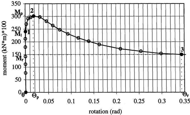
Fig. 7. Internal support test. Moment - rotation graph.
