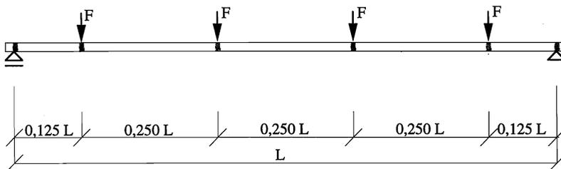
**Fig. 1.** Test set-up for single span tests
