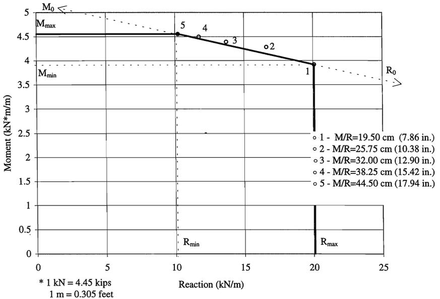
**Fig. 4.** Internal support test. Moment - Reaction (M-R) interaction
