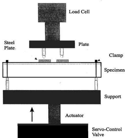
Fig. 4 Test setup for the four-point bending test
