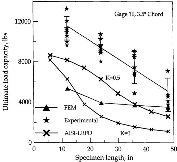
Figure 6. Comparison of the experimental data with the AISI calculations and FEM predictions for gage 16, 3.5" deep C sections.
