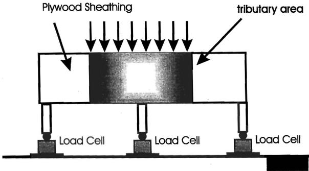
Fig. 9(b) Side view of the three truss assembly system
