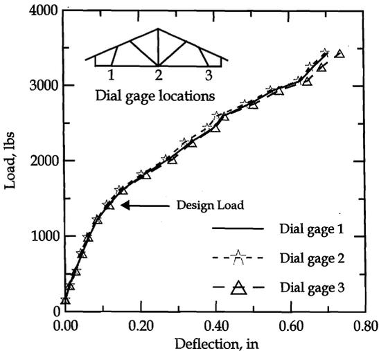
Fig. 10 Bottom chord deflections of the center truss versus load applied on the center truss
