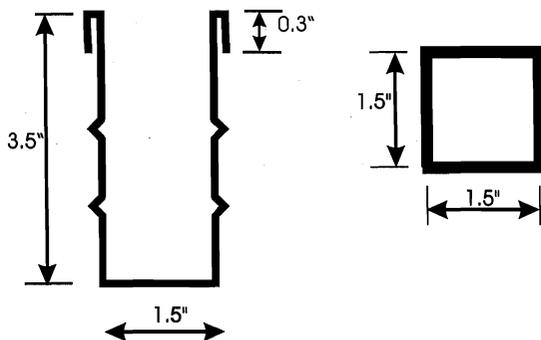
Fig. 1 (a) Typical chord section (designation: 3.5 CHORD 16GA, also available as 2.5" deep section and gages 18 and 20) (b) square section for web and heel section (designation: 1.5 SQWEB 16GA, also available in 18 and 20 gages)
