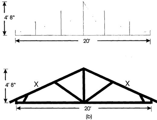
Fig. 7 (a) Initial guess and (b) the lowest cost truss obtained from the optimal design process
