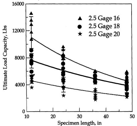
Fig. 3 Experimentally obtained ultimate load (mean value) for the different specimens
