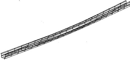
Fig. 5a The first mode of buckling obtained from a linear finite element simulation for axial compression test
