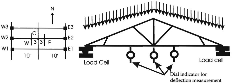
Fig. 9(a) Schematics of the instrumentation of the truss, load cells, and dial gauges
