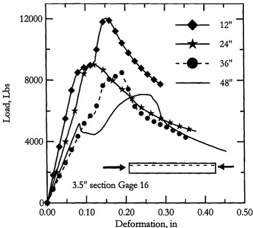
Fig. 2 Load-displacement curve for 2.5 Chord18GA 12"-48" specimens axial compression test
