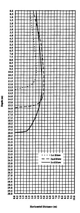
Figure 5(b) Shapes of treatment zones for 2m soft layer and stiff soil plugs
