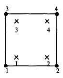
Figure 3 First-order 4-node bilinear axisymmetric quadrilateral finite element
