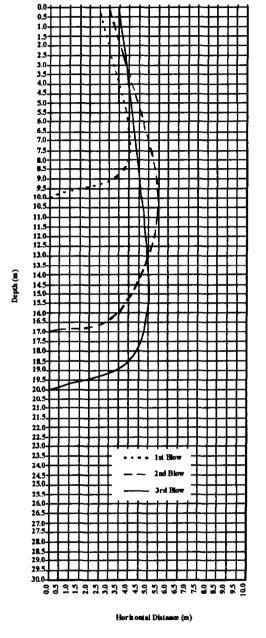
Figure 5(a). Shapes of treatment zones for 1m soft layer and stiff soil plug.
