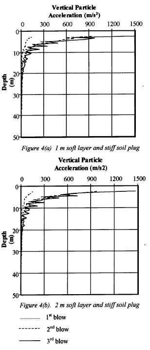
Figure 4 Variations of peak vertical particle acceleration with depth.
