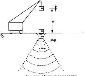
Figure 1 Dynamic compaction
