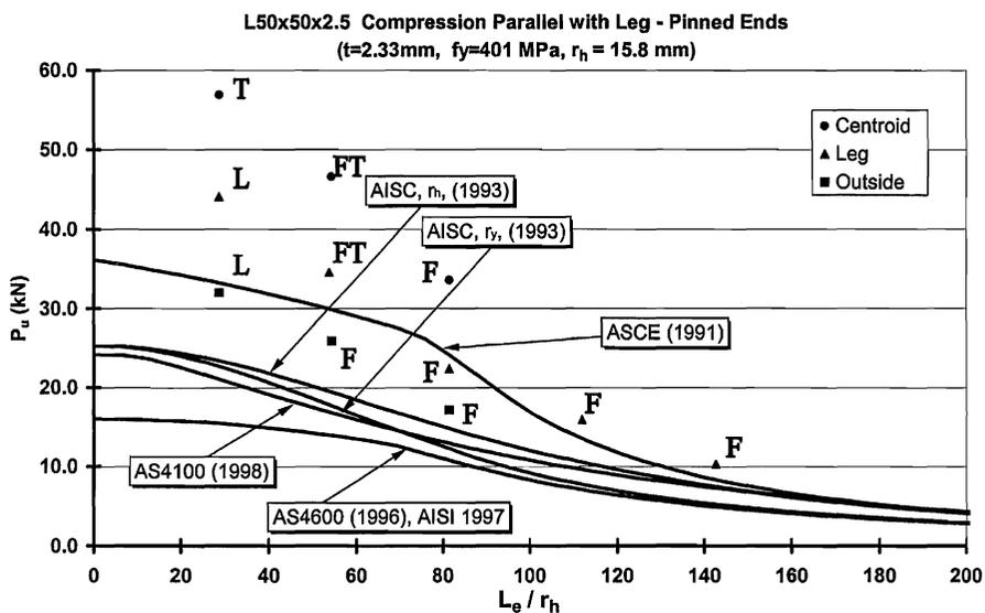
Figure 7: Test strengths vs design curves
