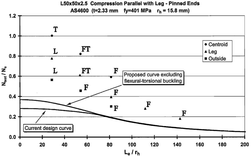
Figure 8: Test strengths vs AS/NZS 4600 and AISI design curves, ( $N_s=56.7$  kN).
