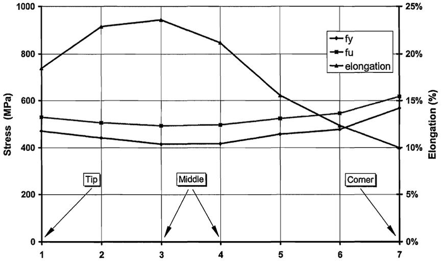
Figure 4: Stress and elongation distribution along leg width
