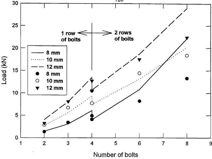
Figure 6 Theoretical and Experimental loads for Type 304 Stainless Steel
