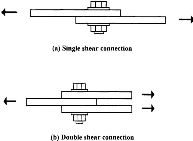
**Figure 3 Single- and Double Shear Bolted Connections**
