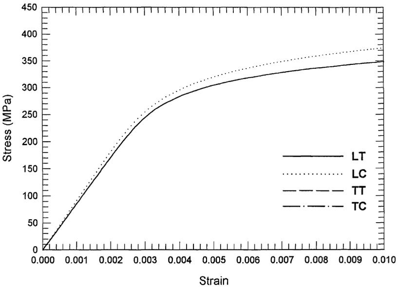
**Figure 2 Analytical Stress Strain Curves for Type 3CR12 Stainless Steel**
