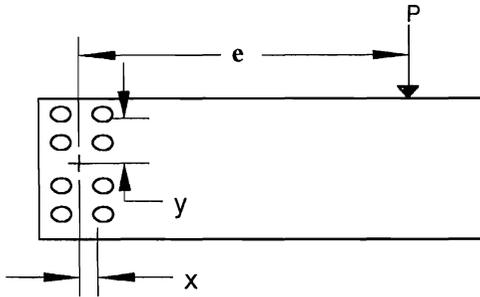
**Figure 4** Detail of Bolted Connection and Applied Load
