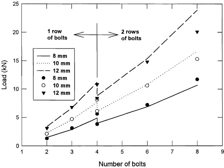
Figure 7 Theoretical and Experimental loads for Type 3CR12 Stainless Steel
