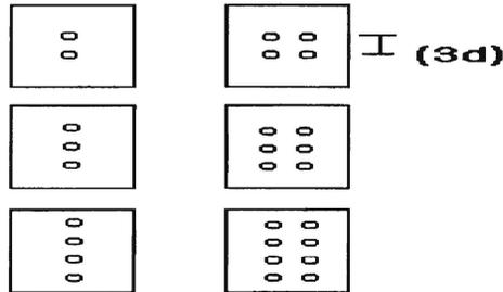
Figure 5 Different bolted combinations
