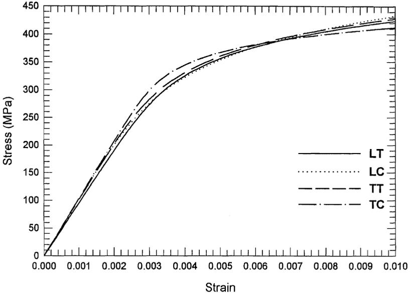
**Figure 1 Analytical Stress Strain Curves for Type 304 Stainless Steel**
