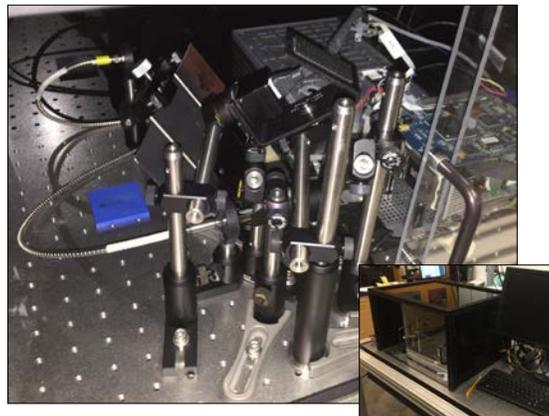
Figure 6. Picture of experimental setup. The inset shows the box containing the entire setup and the desktop computer used to control the laser and the DMD. A second computer was used to control the IR camera.
