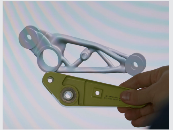
Digital twin of a bell crank for an aircraft (America Makes, Siemens PLM software, One Aviation) (Eckhoff, 2018)
