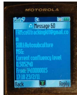
Figure 5. Email and Text Notification. 4 hours prior to reaching the predefined threshold for confluency, an email and text message is sent to alert the human user to prepare for subculture. Once the threshold for confluency is reached, a reminder email is sent. doi:10.1371/journal.pone.0027672.g005
