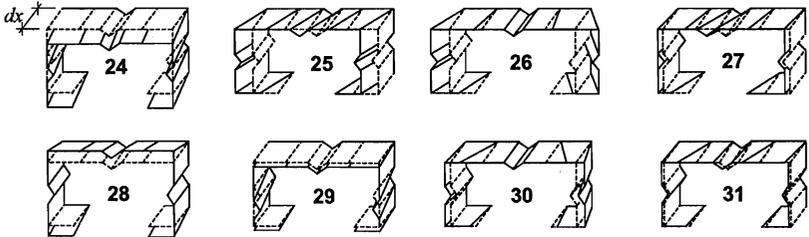
Fig. 4. Stiffened channel 8 most relevant transverse extension modes
