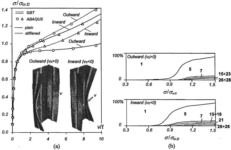
Fig. 7. PFW column distortional (a) post-buckling paths and (b) GBT modal decomposition (stiffened columns)
