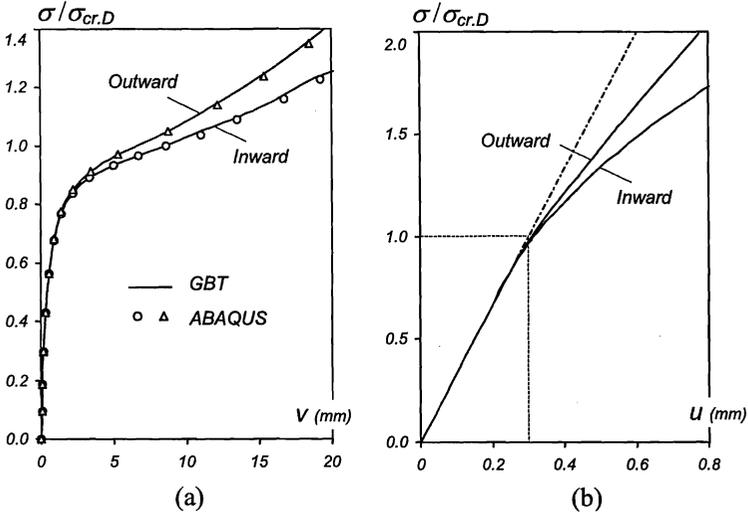
Fig. 10. FWP column distortional post-buckling paths for (a)  $v$  and (b)  $u$  motion: while the PFW curve is practically horizontal, the FWP one exhibits non-negligible slope values.
