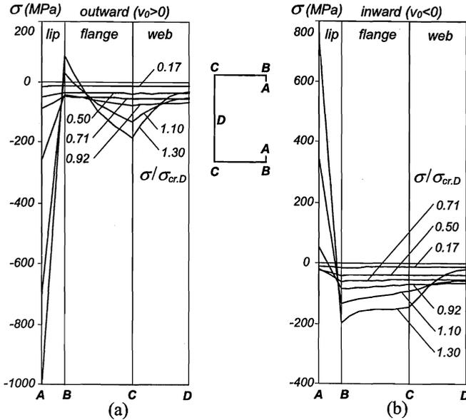
Fig. 8. Plain column mid-span stress distributions: (a)  $v_0 > 0$  and (b)  $v_0 < 0$
