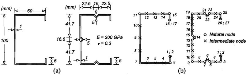
Fig. 1. Lipped channel (a) dimensions and (b) GBT discretizations
