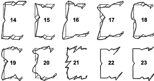
Fig. 3. Stiffened channel 10 most relevant shear modes (warping)
