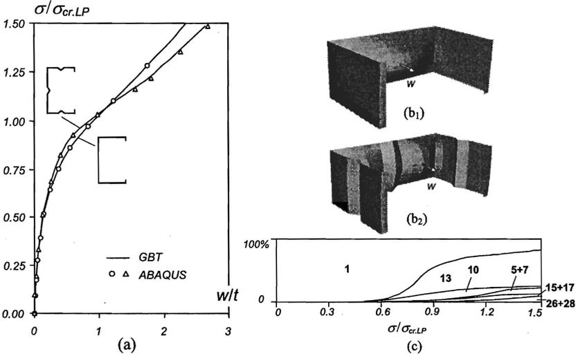
Fig. 6. PFW column local-plate (a) post-buckling paths, (b) deformed configurations and (c) GBT modal decomposition (stiffened column)
