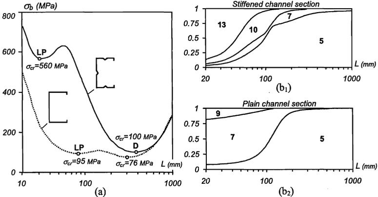
Fig. 5. Plain and stiffened channel PWF columns: (a) single-wave  $\sigma_b$  vs.  $L$  curves and (b) GBT modal analysis of the buckling modes
