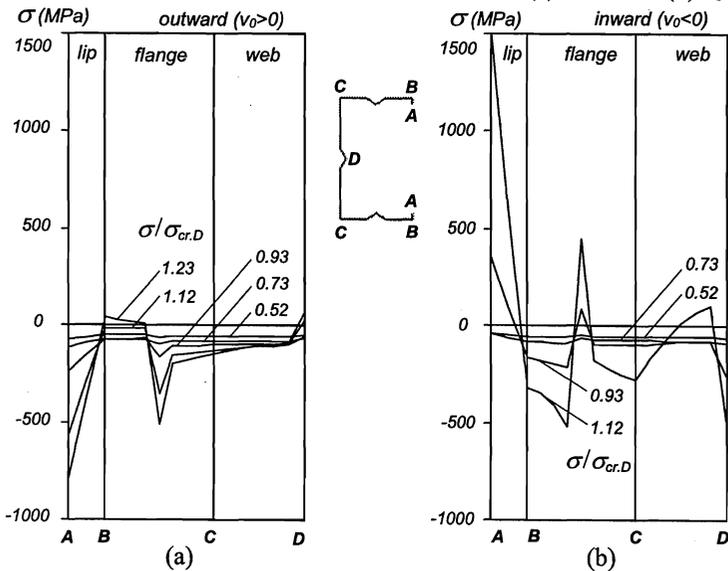
Fig. 9. Stiffened column mid-span stresses: (a)  $v_0 > 0$  and (b)  $v_0 < 0$
