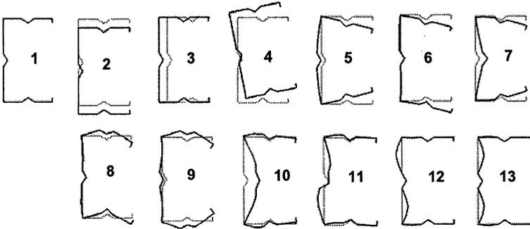
Fig. 2. Stiffened channel 4 global, 7 distortional and 2 local-plate modes
