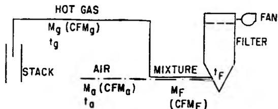
FIG. 1: DILUTION WITH AMBIENT AIR
