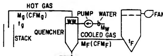
FIG. 2: EVAPORATIVE COOLING
