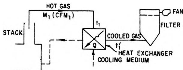
FIG. 4: A HEAT RECOVERY SYSTEM
