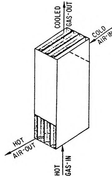
FIG. 9: PLATE TYPE HEAT EXCHANGER
