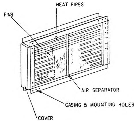
FIG. 7: HEAT PIPE HEAT RECOVERY UNIT
