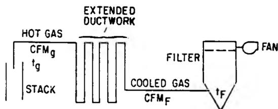
FIG. 3: NATURAL CONVECTION AND RADIATION
