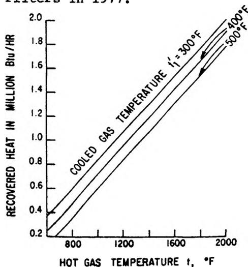
FIG. 5: APPROXIMATE HEAT REMOVAL FROM 1000 SCFM OF A GAS
