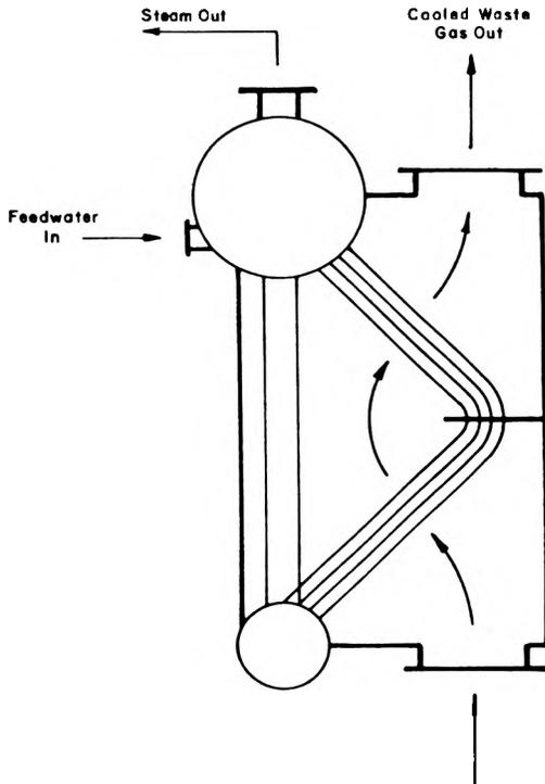
Figure 3. Waste Heat Boiler
