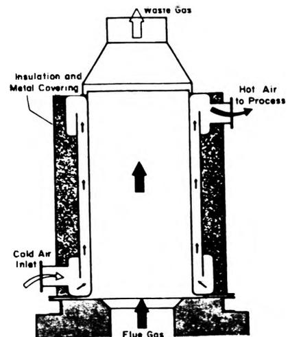
Figure 5. Metallic Radiation Recuperator
