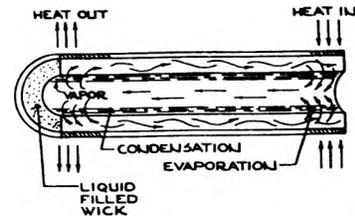
Figure 4. Heat Pipes
