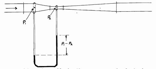
This meter effects the measurement of air in essentially the same manner as the orifice meter, but owing to the long tapering case on the down-stream side, the formation of eddies are avoided, and a very much larger proportion of the pressure drop  $(P_1 - P_2)$  is recovered. This discharge formula for the Venturi tube is of the form:
