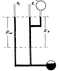
$P_1 =$  Pressure inside drum. ZW = Inches of water. Zo = " Oil. WZW = Weight of water column. OZo = " " oil ".
