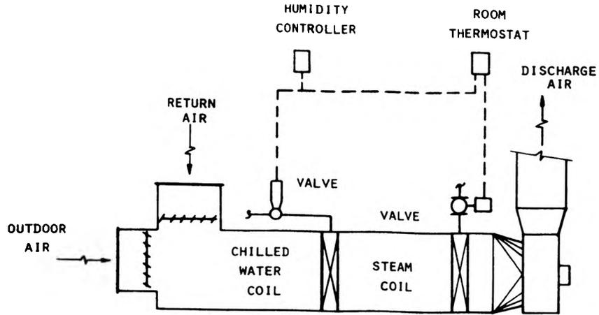
FIGURE 4. WORKSPACE AIR HANDLING SYSTEM
