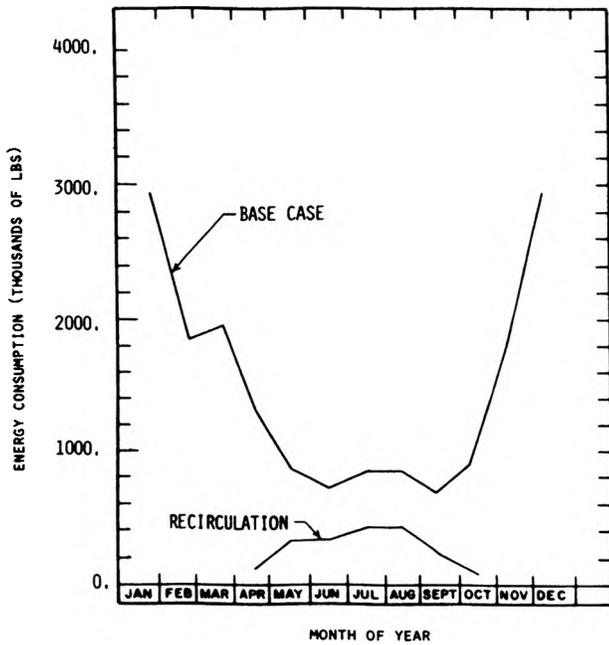
FIGURE 5. PREDICTED HEATING ENERGY CONSUMPTION (STEAM)
