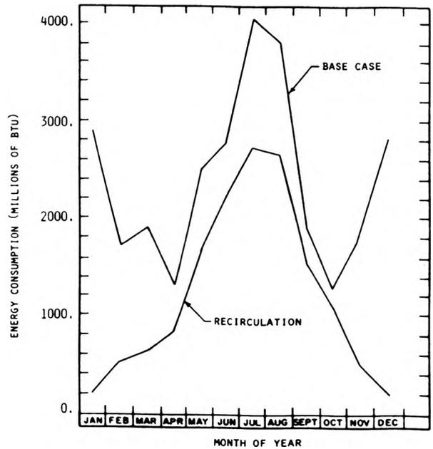
FIGURE 3. TOTAL HEATING AND COOLING ENERGY REQUIREMENTS
