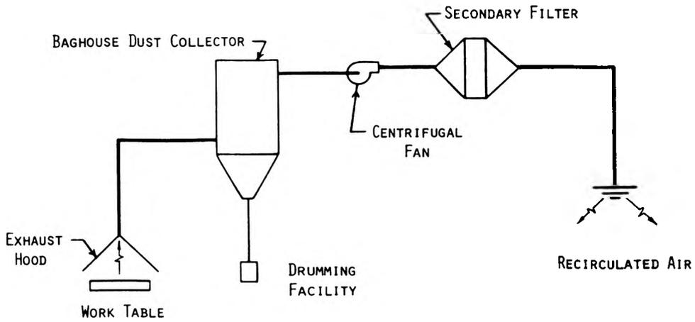
FIGURE 1. RECIRCULATION SYSTEM SCHEMATIC
