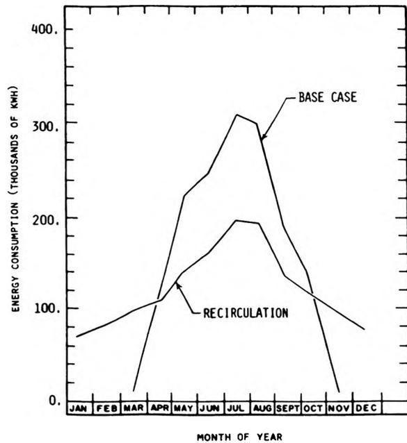
FIGURE 6. PREDICTED COOLING ENERGY CONSUMPTION (ELECTRICITY)
