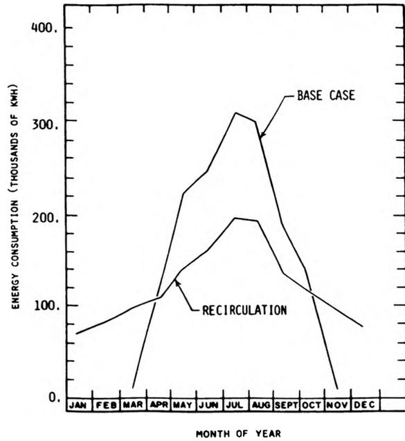
FIGURE 6. PREDICTED COOLING ENERGY CONSUMPTION (ELECTRICITY)
