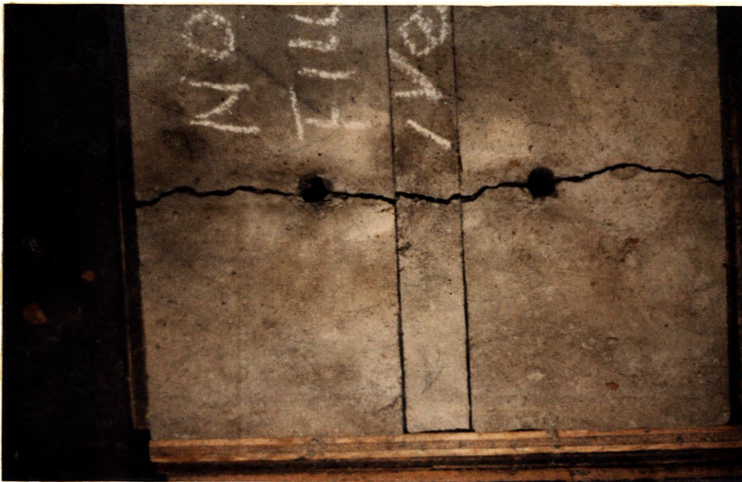
Figure D-6: Two Closed Joint Concrete Model Test: Test C-12, S=3 7/8 in., A Success
