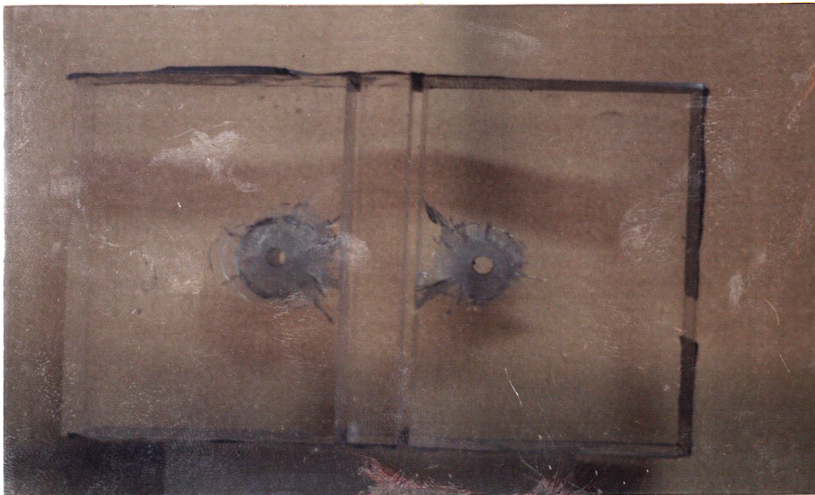
Figure E-22: Post-test Picture of the Test No.4, Showing the Cratering Effect in the 1/4 in. Sand Filled Two-Joint Plexiglas Test
