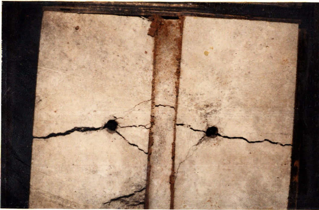
Figure D-15: 1/8 in. Clay Filled, Two-Joint Concrete Model Test: Test C-35, S=3 3/4 in., A Success
