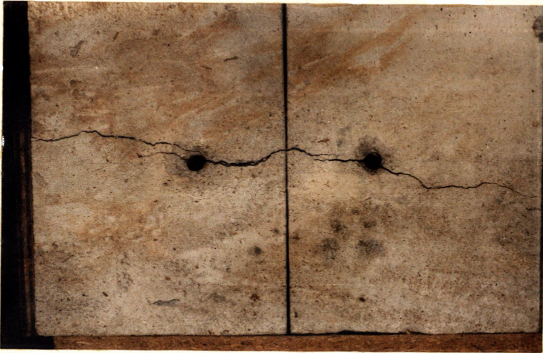
Figure D-3: Single Closed Joint Concrete Model Test: Test C-6, S=4\frac{1}{2} in., A Success
