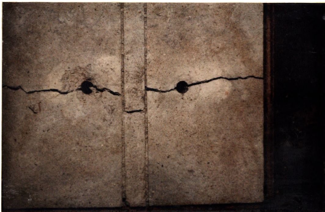
Figure D-10: 1/8 in. Sand Filled, Two-Joint Concrete Model Test: Test C-19, S=3 \frac{3}{4} in.
