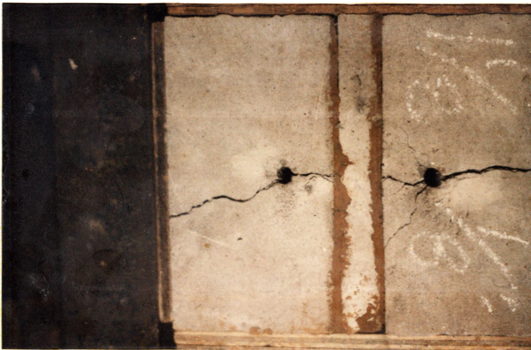
Figure D-16: 1/8 in. Clay Filled, Two-Joint Concrete Model Test: Test C-36, S=3 7/8 in., A Failure
