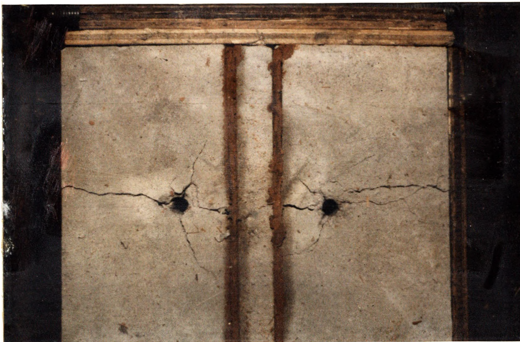
Figure D-17: 1/4 in. Clay Filled, Two-Joint Concrete Model Test: Test C-39, S=4 in., A Failure
