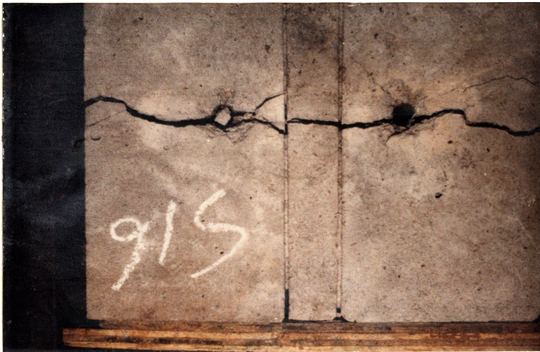
Figure D-8: 1/16 in. Sand Filled, Two-Joint Concrete Model test: Test C-16, S=3 7/8 in., A Success
