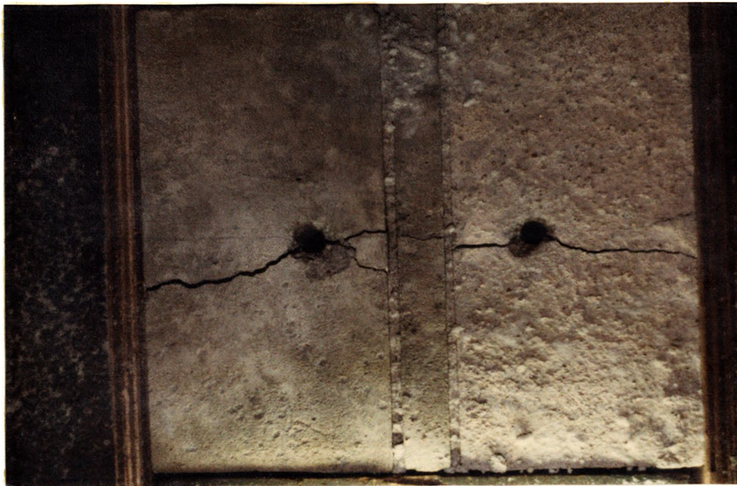
Figure D-12: 1/4 in. Sand Filled, Two-Joint Concrete Model Test: Test C-24, S=3 5/8 in., A Success
