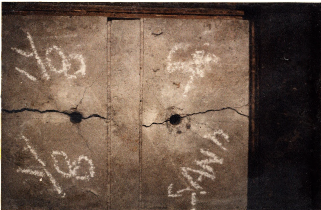
Figure D-9: 1/8 in. Sand Filled, Two-Joint Concrete Model Test: Test C-21, S=3 \frac{7}{8} in., A Failure.
