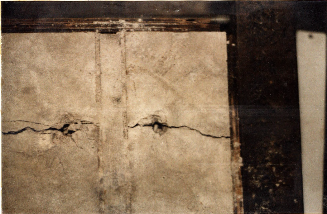
Figure D-11: 1/4 in. Sand Filled, Two-Joint Concrete Model Test: Test C-22, S=4 1/4 in., A Failure.
