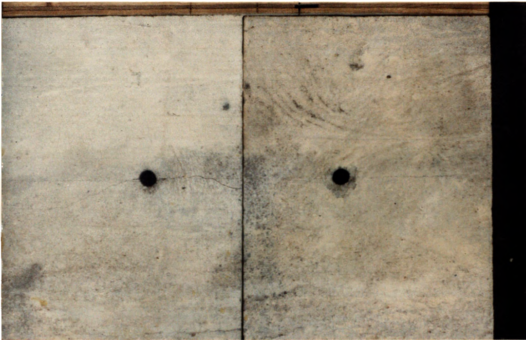
Figure D-4: Single Closed Joint Concrete Model Test: Test C-7, S=5\frac{1}{4} in., A Failure
