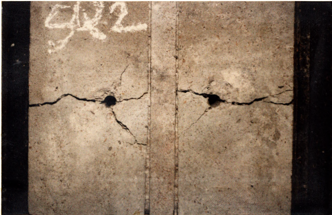
Figure D-22: 1/8 in. Sand Filled, Two-Joint Concrete Model Test: Test C-19, S=3\frac{3}{4} inch, Cratering Occurred from Boreholes to Discontinuities
