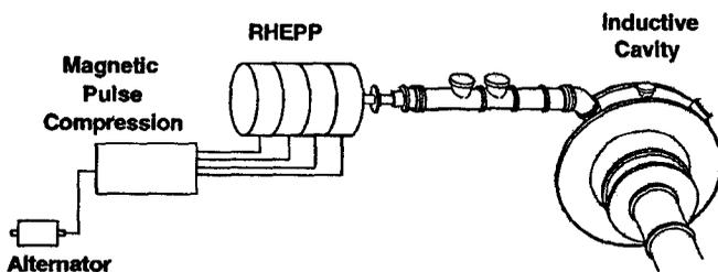
Figure 3. The ETF pulsed power concept
