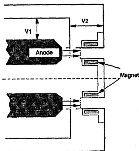
Figure 5. The two-stage extraction ion diode concept
