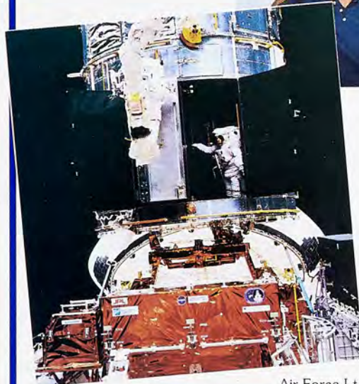
Above: Tom Akers maneuvers inside the bay which will house the Corrective Optics Space Telescope Axial Replacement (COSTAR) while assisting Kathryn Thornton (partially visible at left) with the installation of the 640-pound instrument.
