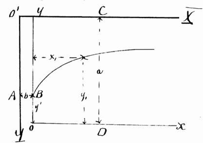
Let A = b = distance of  $\underline{Y}$  axis from y and C = a = distance of  $\underline{X}$  axis from x.
