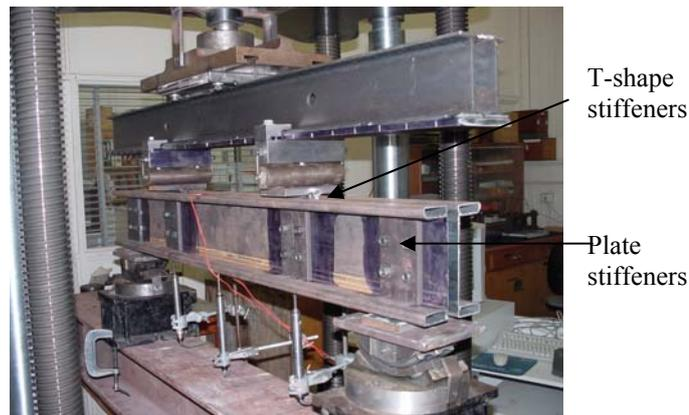
**Figure 5. Section Capacity Test Rig**
