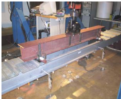
Figure 2 Distortional buckling test
