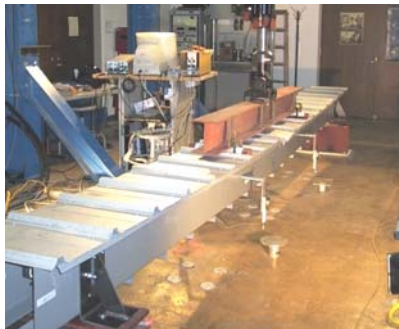
Figure 1 Local buckling test
