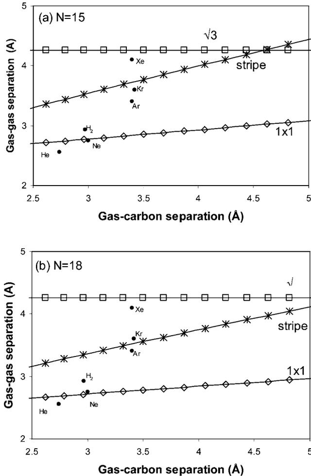
FIG. 2. Resulting gas-gas separation and gas-carbon separation as the distance between the NT and adatom is varied, for  $N=15$  and  $N=18$  tubes. The lines represent the limiting (shortest) distances for the various phases, as shown. Also plotted are  $\{\sigma_{gC}, \sigma_{gg}\}$  for the various gases. The relative phase stability can be estimated from these curves, as discussed in the text.
