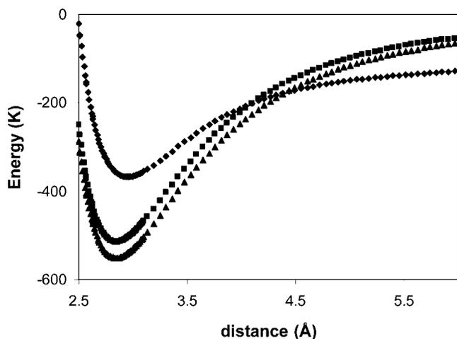
FIG. 3. Adsorption energy of  $H_2$  as a function of distance  $d$ , for the case of an  $N=18$  tube. Curves represent results for the  $1 \times 1$  phase (diamonds), the  $\sqrt{3}$  phase (squares), and the striped phase (triangles).
