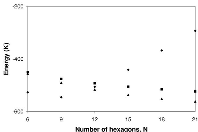
FIG. 4. Adsorption energy for  $H_2$  as a function of  $N$ . Symbols as in Fig. 3.
