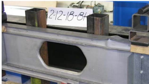
Figure 5 - Photograph of Typical Flexural Failure of iSPAN Joist
