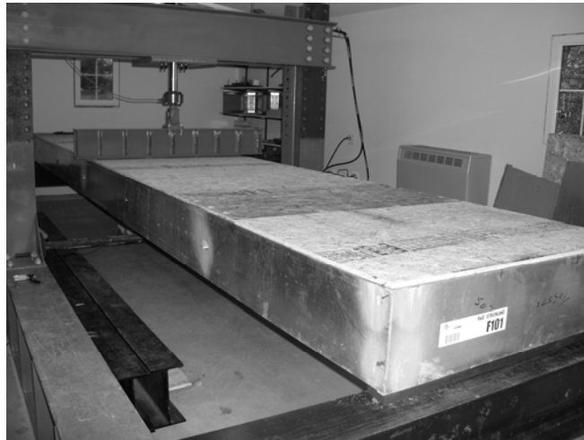
Figure 9 C-section Floor in Test Frame
