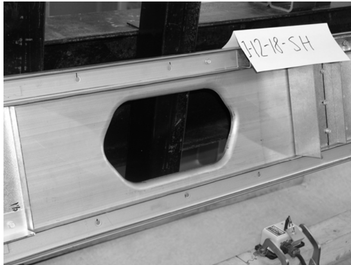
Figure 6 - Typical Shear Failure WITH Holes
