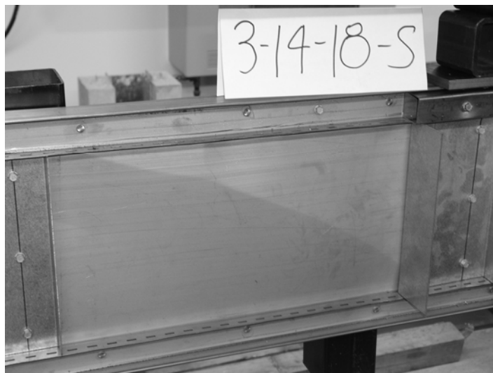
Figure 6 - Typical Shear Failure WITH Holes
