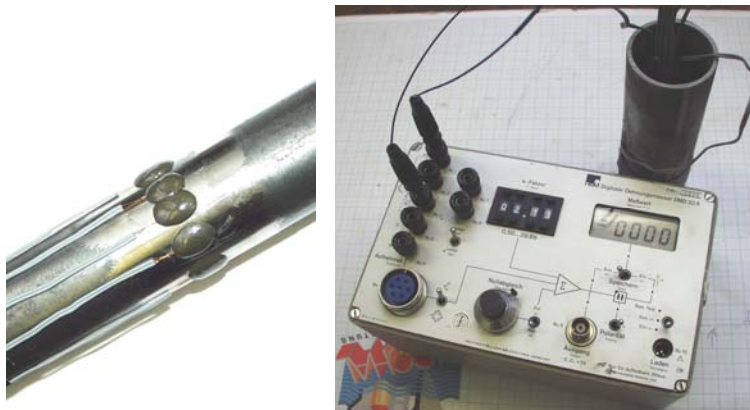
Figure 4: Applied strain gages and measuring device
