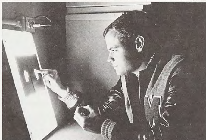
A student inspects an industrial radiograph in the nondestructive testing lab.
