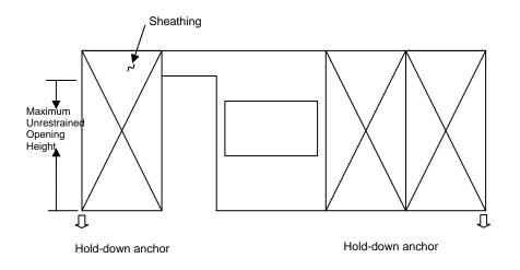
**Figure 7.** Type II (Perforated) Shearwall (Sputo and Turner, 2006) **Chapter 3 - Cold-Formed Steel in Metal Building Systems**
