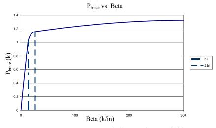
Figure 3. Relationship Between  $P_{\text{brace}} \, vs \, \beta \,$  (Sputo and Turner, 2006)
