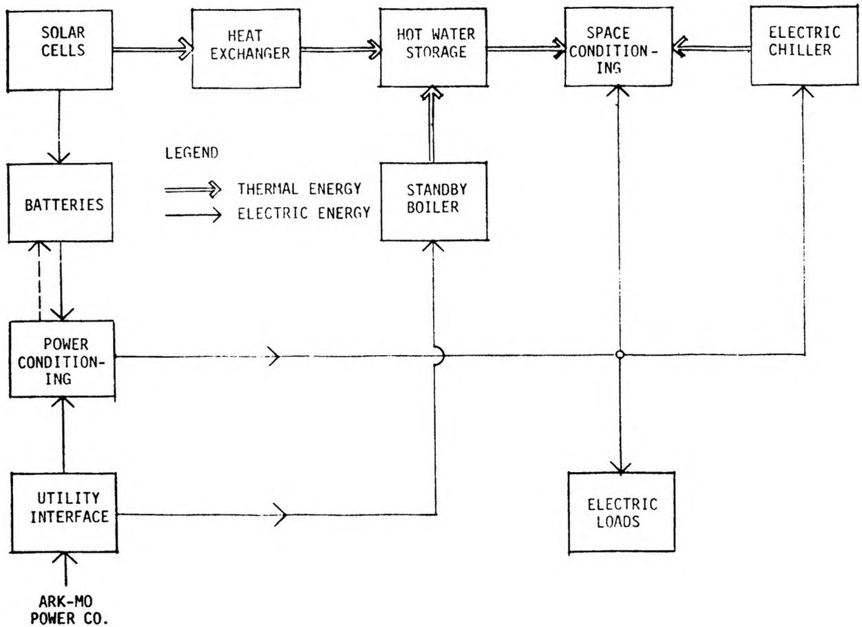
FIGURE 1. SIMPLIFIED SYSTEM SCHEMATIC DIAGRAM
