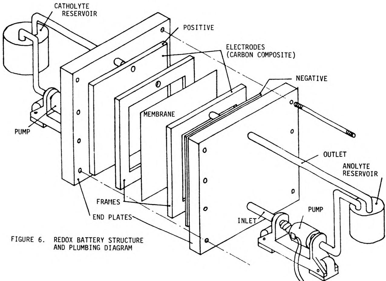
FIGURE 6. REDOX BATTERY STRUCTURE AND PLUMBING DIAGRAM
