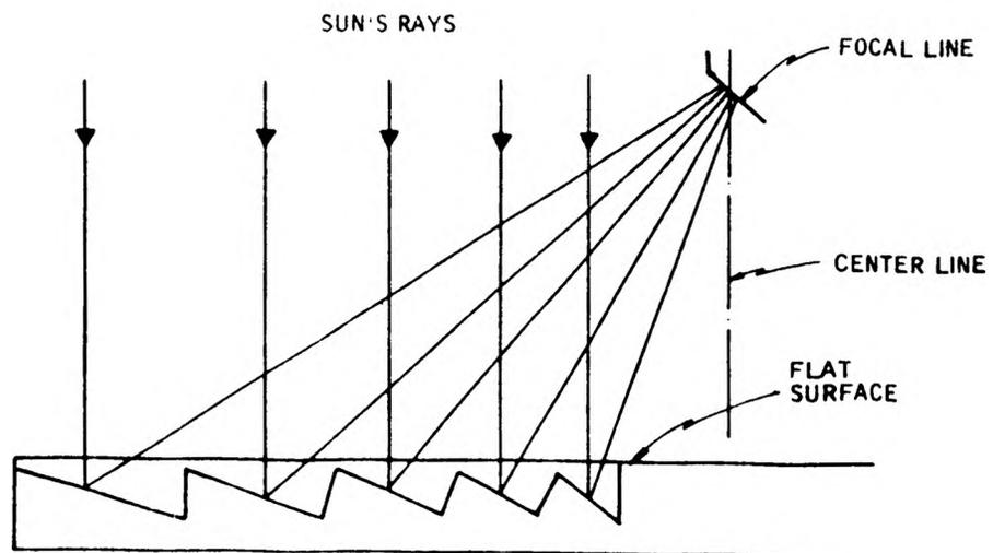
FIGURE 2. SECTION OF FACETED SECOND SURFACE REFLECTOR
