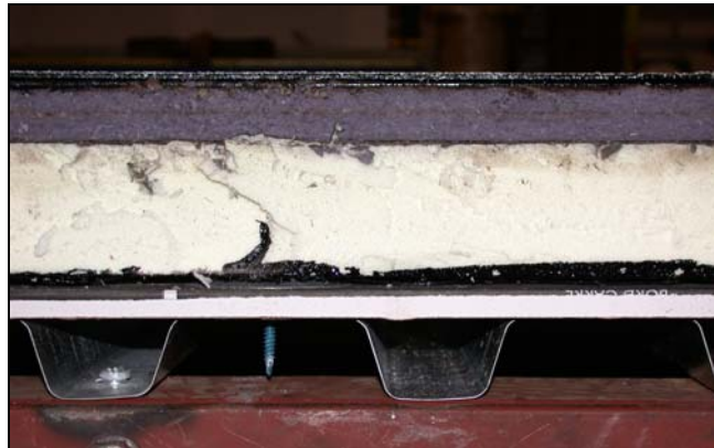
Figure 1 : SBS-34 roofing cross-section as tested by Yang (2003)
