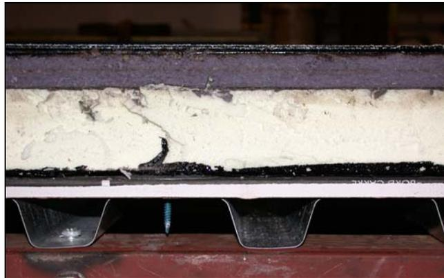
Figure 1 : SBS-34 roofing cross-section as tested by Yang (2003)
