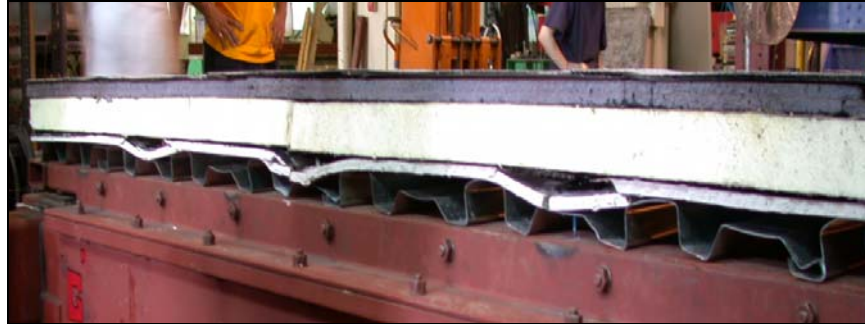
Figure 5: Warping deformation of steel deck restrained by non-structural components – test 45 (Yang 2003)
