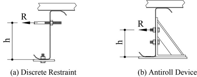
Figure 2 Restraint Devices
