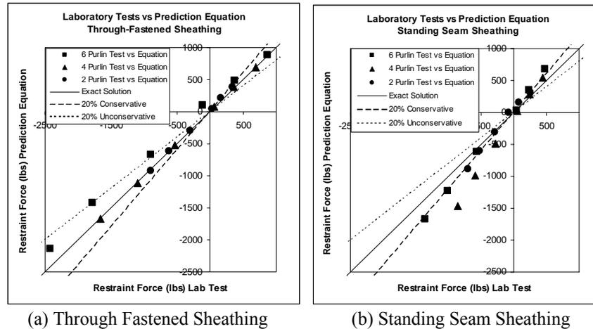
Figure 6 Comparison of Prediction Equation with Laboratory Tests
