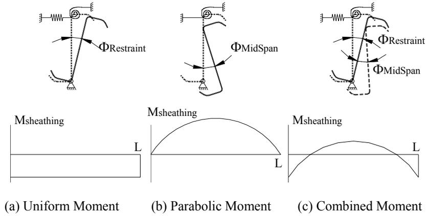
Figure 4 Sheathing Moment - Z-section with Flexible End Restraints
