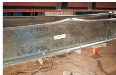
(b) unrestrained 800S200-054 C exhibiting distortional buckling
