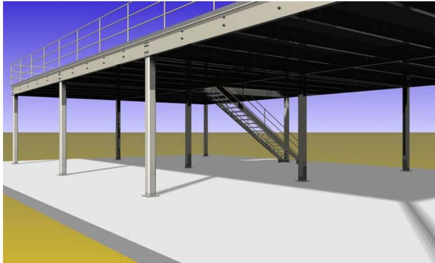
FIGURE 2 – TYPICAL CFS-SBMF USED AS INDUSTRIAL PLATFORM MEZZANINE
