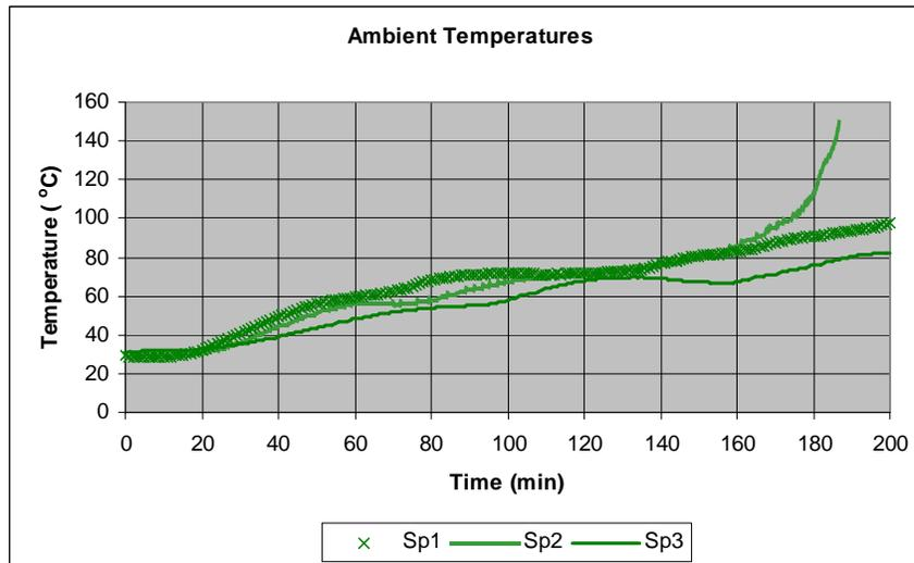
Figure 13: Ambient Side Time-Temperature Profile of Specimens 1, 2 and 3
