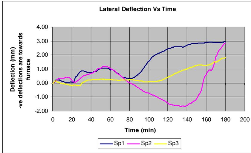
Figure 12: Lateral Deflection-Time Profile of Specimens 1, 2 and 3
