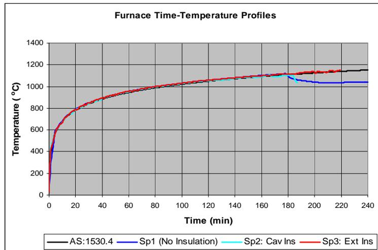
Figure 7: Furnace Time-Temperature Profiles for Test Specimens 1, 2 and 3
