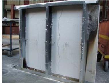
Figure 4: Failure of Test Specimen 1 built without insulation
