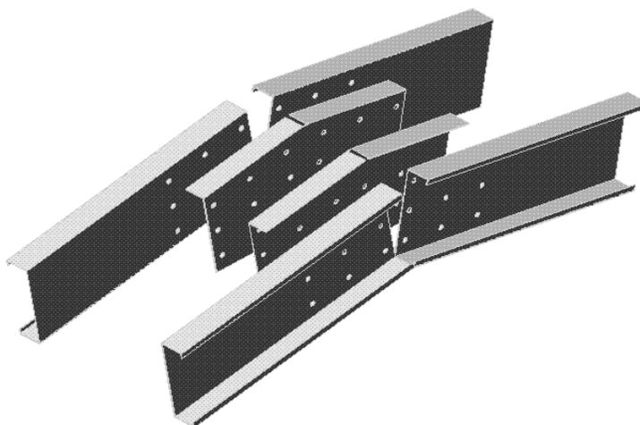
Figure 1. Details of typical bolted moment connection
