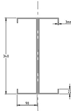
Figure 6. Dimensions of channel-section used in parametric study
