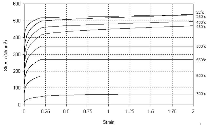
Figure 2. Stress-strain curves at different temperatures
