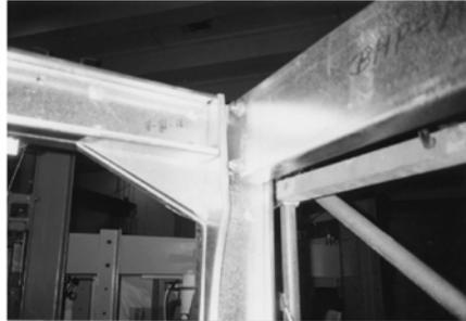
Figure 4. Typical web buckling induced failure [Ref. 14]
